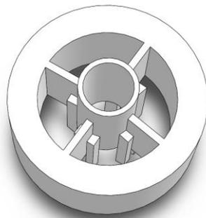
**Figure 19 Illustration of 3D-printed skeleton part**
