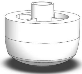
**Figure 18 Illustration of 3D-printed bottom part of male connector**
