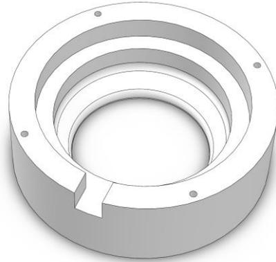
**Figure 28 Illustration of the 3D-printed plastic part where the security ground ring is mounted**
