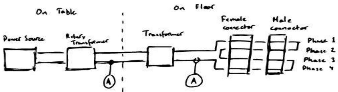
Figure 32 Illustration of the test rig
