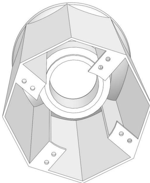
**Figure 25 Illustration of female connector housing**
